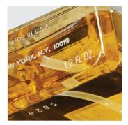
Ideal overt codes are permanent to prevent removal by unauthorized parties. Laser marking systems can provide high quality permanent codes on many package types.
